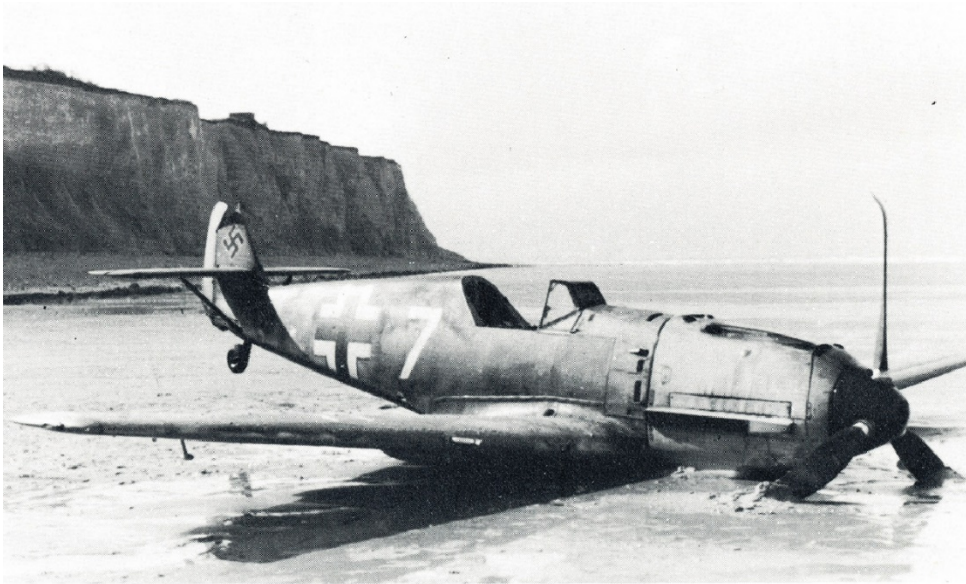
Figure 5 - The fate many Bf109s suffered during the Battle of Britain due to battle damage or fuel starvation. Internal fuel of 88gal/400L only gave the Bf109E-3 and E-4 a maximum of 10-20 mins over England. As a result, a number of returning 109s ditched in the English Channel or crash landed in France. The arrival of the E-7 variant with a 300 l / 68 gal alloy drop tank came too late to have any influence.
