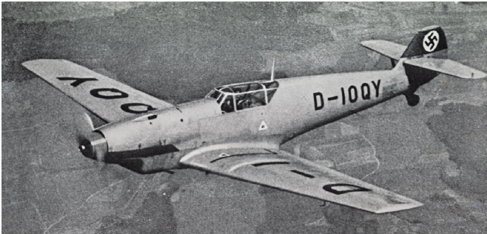
Figure 3 - Bf109V 4 (V=Versuchs / test aircraft). Armed with three MG 17, 7.92 mm machine guns, the third fired through the propeller hub.
